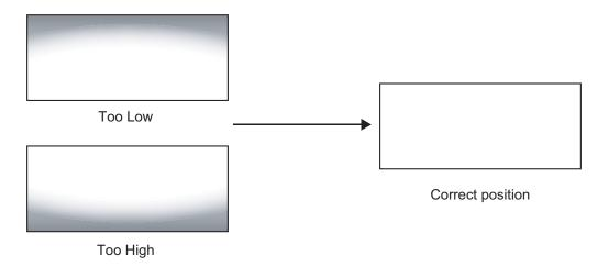
When the height is properly set, tighten the Height Adjustment T-Screws to secure the lens in place.
